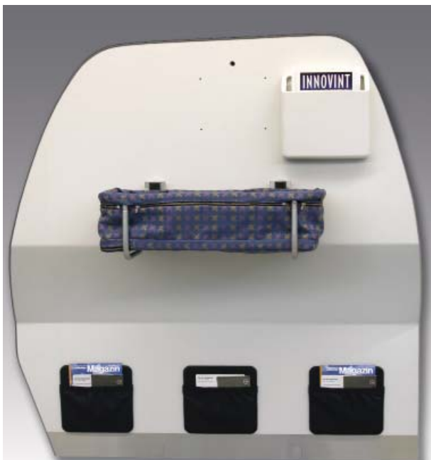
Baby Bassinet installation • with fittings PNR 1600-series
