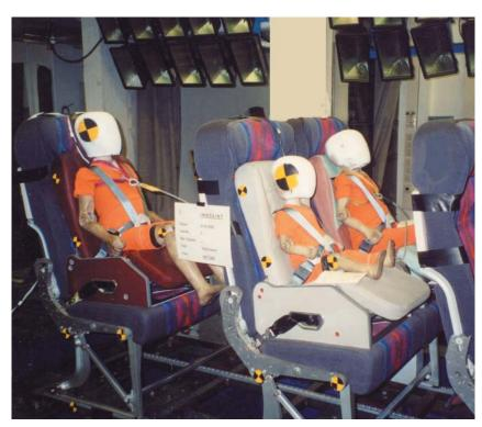
CRS – Child Restraint System • 16g dynamic test SAE AS 8049 with CRS FWD–Installation
