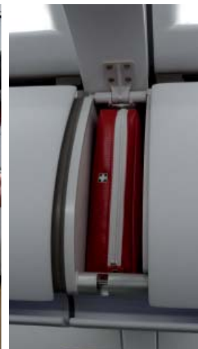
PNR 6240-87S • First Aid Kit stowed in A320 CAS headrest and hatrack lifeline spacer
