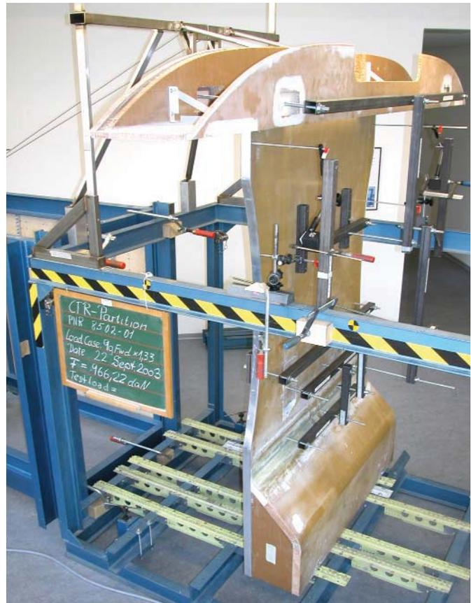
Universal test jig for static testing with loads up to 5 t
