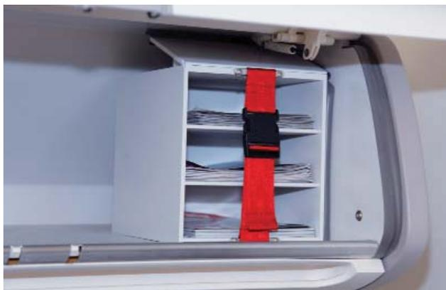
Overhead Stowage Magazine Rack • shown without divider panel
